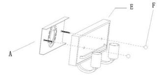
Step 2: Carefully pass wires from outlet box through back plate (A)
