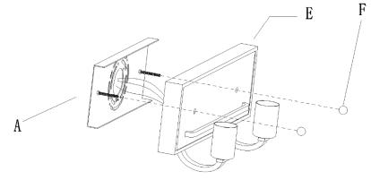
Step 5: Install bulb (Not included. Please do not exceed the maximum capacity recommended on the socket.)
