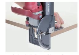
**Vertical stability** by attaching to the baseplate to increase the surface
