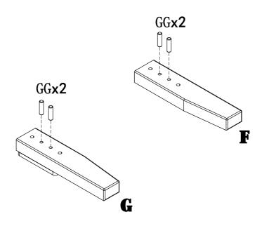
**2.**Take out the left sideboard (H) and right sideboard (I) and insert wood dowel (GG) into the side two holes as shown photos.
