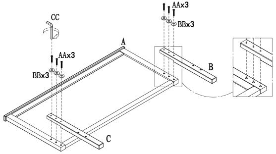
**4.**Turn assembled headboard over,fasten the headboard support bar(D) to the 2 holes in leg(B and C) with screw(DD) fitted with washer(BB).Use allen key(CC) to drive(DD).
