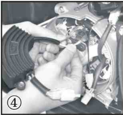
④ Take down the AVR from carbon-brush
