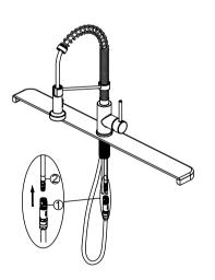
Push the quick connector (1) firmly upward and attach it to the receiving block (2). Pull down moderately to ensure the connection has been made.
