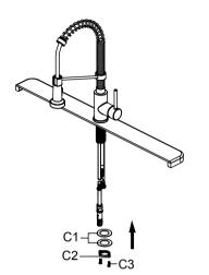
Install the rubber washer and metal washer (C1) onto the threaded mounting shank. Thread the nut (C2) onto the mounting shank. Lock the nut (C2) into position by tightening the screws (C3). Do not overtighten.
