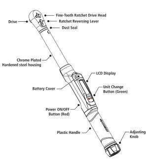
**WARNING:** DO NOT turn the adjusting knob either below the lowest scale reading or above the highest scale reading. The LCD display will show torque settings beyond the calibrated upper and lower limits of your torque wrench, these are intended for adjusting purposes only and are not within the calibrated range.
