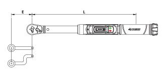
E – Effective Length of extension measured along the center line of the torque wrench
