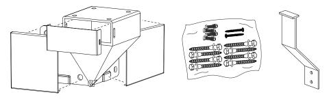
**4.** Starting at one end of the railing, hold the first fascia mount bracket in position ensuring that the top of the bracket is level with the deck surface. Mark the position of the 8 fastener holes on the fascia boards.
