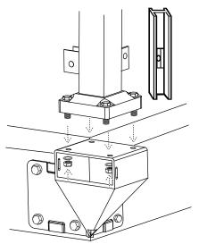
**9.** Attach remaining brackets to deck structure following steps 3-6 above.
