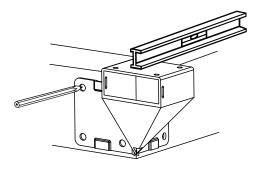
**5.** Remove the bracket and drill 3/16" pilot holes at the marked positions.
