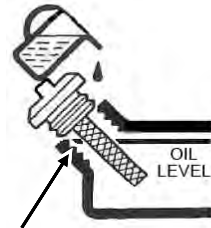
Figure 2 - Add Oil To TOP Of Threads
