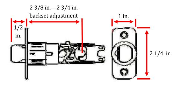
Can be adapted for radius-corner, square-corner or circular drive-in applications
