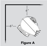
Placement near a wall or corner Please position at least 6" away from walls or other large surfaces. Doing so will ensure your Tower Circulator has adequate room to intake air, providing optimum performance. (See Figure A)
