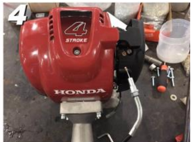
Connect accelerator cable to engine.
