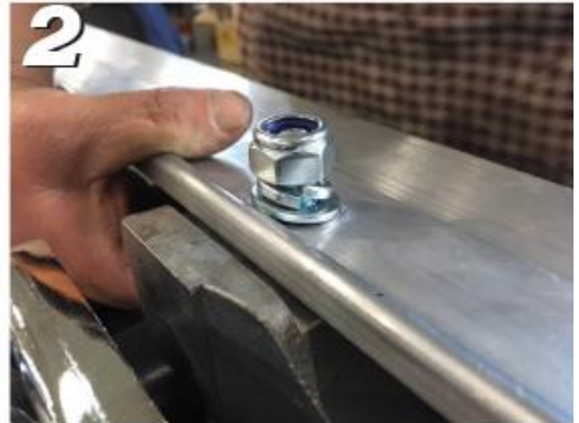
Attach washers, locking screws, and bolts.
