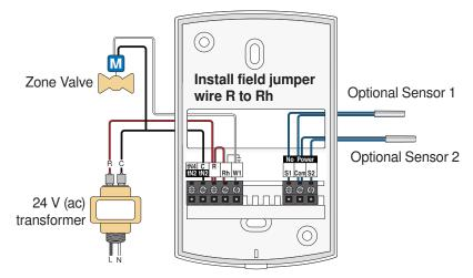
Wiring - Stand Alone to Switching Relay or Zone Valve Control
