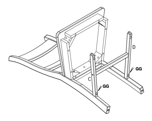
**5** Use screw(GG) to fasten left leg(F) and right leg(G)to side rails(C&D)
