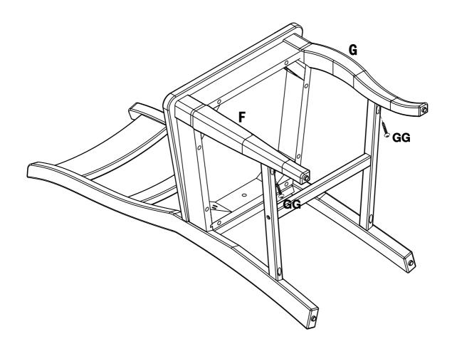
6 Use allen key(DD) to tighten left leg(F) and right leg(G)to the seat panel(B) with screw(EE) and washer(BB&CC)
