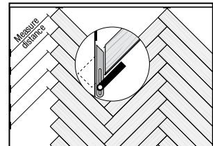
**NOTE:** To cut a plank, simply measure and mark the plank. Then, use a straight edge and utility knife to score and snap. You will also need to back-cut the under pad on the bottom of the plank. If you have difficulty using this method, you can use a jig saw, circular saw or miter saw.
