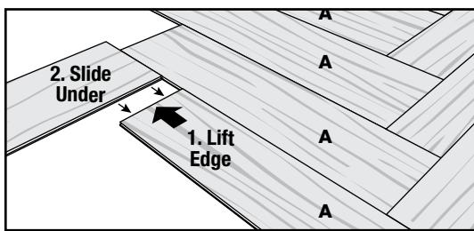
Position the tongue and groove of the first plank in column A2 into place with the last plank in column B1. Tap seams to completely lock planks.
