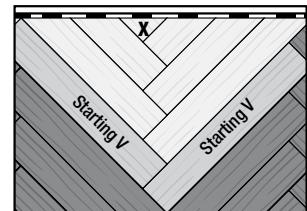
When finishing the floor with small triangular shaped pieces (see plank X), use a small bead of "instant glue" (cyanoacrylate adhesive) in the groove before tapping in the plank. Remove any excess adhesive as soon as possible using mineral spirits.
