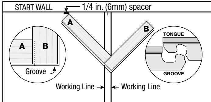
**Note:** Top décor edges should be flush with no high spots (run your hands over the plank seam, tap down as necessary.)
