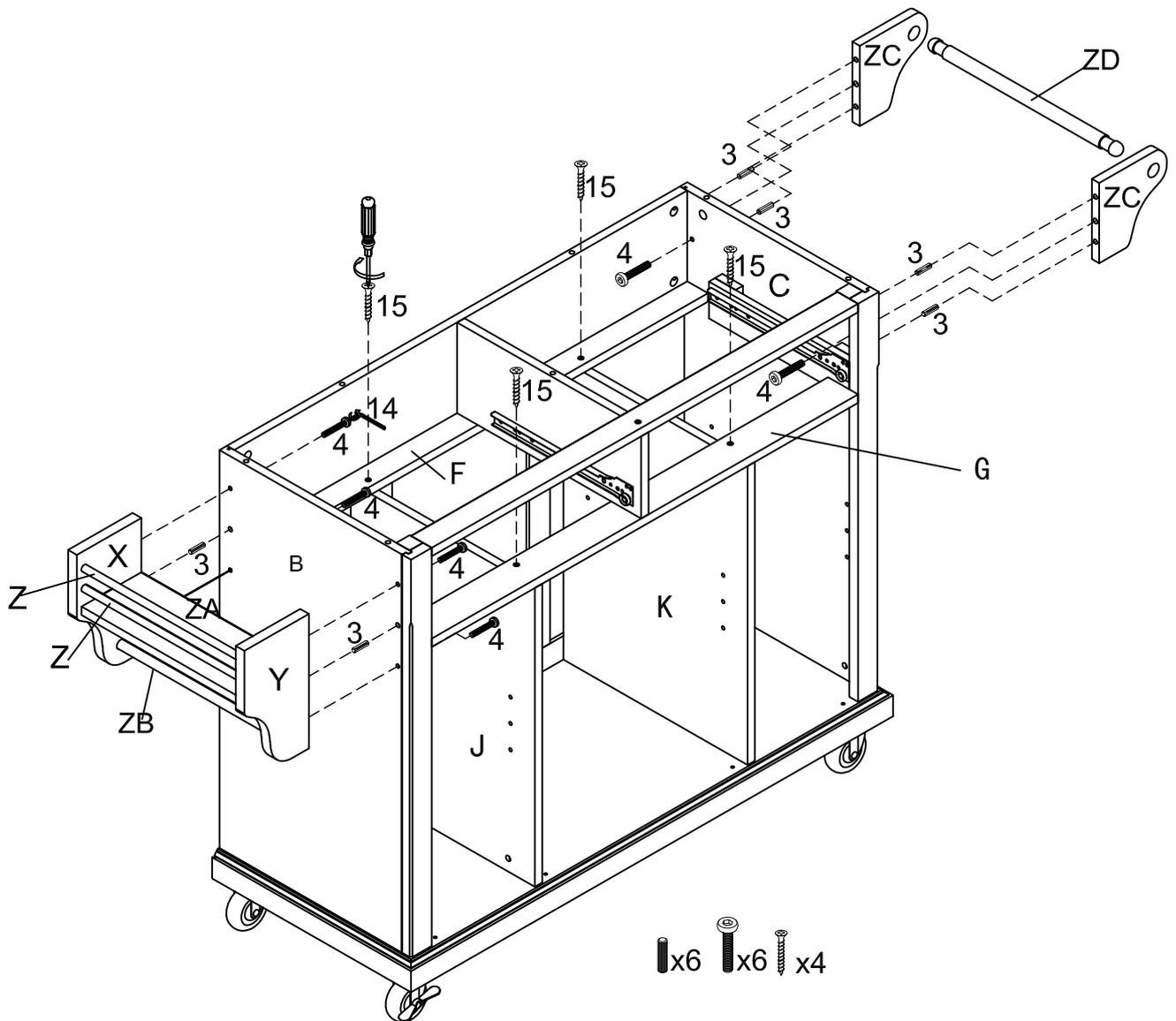
**Step 11. Attach Top A to cabinet using Wood Dowels & Cam locks as shown.**
