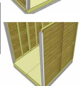
**22.** Attach Door Jamb to vertical wall stud with 4 - 2 1/2" screws. Complete both Door Jambs.
