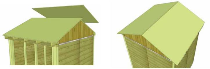
**45.** Locate Plywood Roof Piece for the rear side (78" x 45 1/4").
