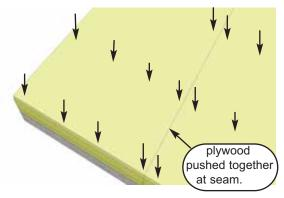
**11.** With Plywood positioned correctly on floor framing, attach using 16 - 1 1/4" screws per sheet.
