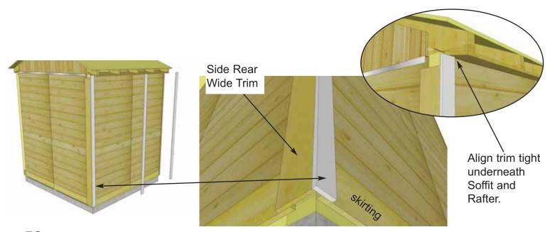
**52.** Attach **Narrow Trims** (**Rear Walls**) to in each rear corner and middle wall seam (3 - 1/2" x 2 1/2" x 79"). Use 8 - 1 1/2" finishing nails per piece. Align Trims tight underneath Soffit and Rafter and so it caps the Side Rear Wide Trim.
