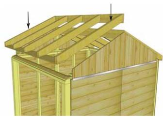
**38.** Place 2nd completed Rafter Section on gable wall framing. Position as per **Steps 34 - 36.**
