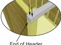
End of Header flush with outside of Door Jamb.
