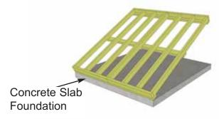
9. With Floor Runners attached, carefully flip the floor over and place on your foundation.
