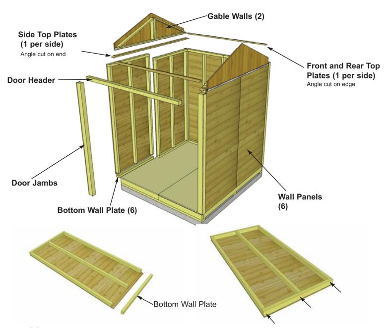
**12.** Starting with **Solid Wall Panels**, carefully lay panel face down. Position and attach **Wall Plate** to bottom of wall studs of each wall panel with 3 - 2 1/2" screws. Position plates flush with framing.
