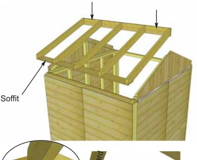
**35.** Starting at the rear, lift a completed rafter section up and place on gable framing.
