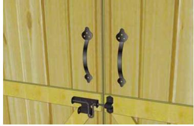
**68.** Attach **Door Handles**. Handles are positioned on top section of each door and mounted with 3/4" Black Screws.
