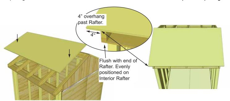
**43.** Starting in front corner, locate 5/8" x 78" x 45 1/4" Plywood Roof Section and place on top of Roof Rafters. Position so Plywood overhangs outside Rafter by 4". At bottom of Rafter, Roof Panel should be flush with Rafter end.
