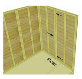
**19.** Align wall panel framing flush with floor framing and attach vertical wall studs together as per **Step 18.**
