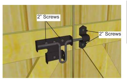
**67.** Attach Black Barrel Bolt as illustrated above with 2" & 3/4" Black Screws. Note how female part of Barrel Bolt is positioned higher than male. Do a dry run first to position Barrel Bolt correctly. **Important** - Drill a shallow pilot hole with 1/8" drill bit prior to securing with screws to prevent wood splitting.
