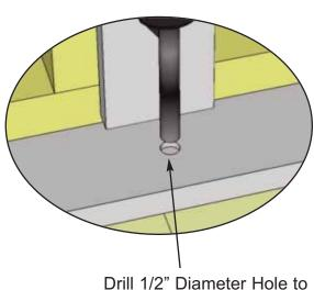
Drill 1/2" Diameter Hole to accommodate rod of Cane Bolt.
