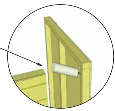
**16.** Position side wall into place on plywood floor. Butt both vertical wall studs of side and rear walls together and attach with 3 - 2 1/2" screws. Screw at the bottom, middle and top of stud to secure properly.
