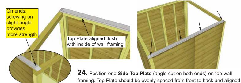
flush with the inside of wall framing. Attach into wall framing with 4 - 2" screws.
