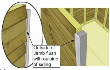
**21.** Locate Door Jambs. Align so attached filler strip is facing to the outside. Position outside of Jamb flush with outside of siding. At the floor, Jamb should be flush with
