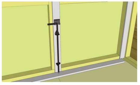
**66.** The Interior Cane Bolt will be attached to Vertical Door Flange. To position Cane Bolt correctly, attach to flange first, close doors and mark hole to house Cane Bolt Rod. Open doors and drill hole where previously marked with 1/2" bit. Attach with 3/4" Black Screws.
