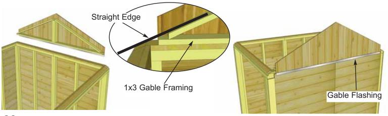
**28.** Place Gable so framing sits flush with the inside of the top plate. Center from front to rear using a Straight Edge to confirm angle of gable frame and Top Plate line up. Adjust gable accordingly. From the outside, make sure gable flashing overhangs wall siding.
