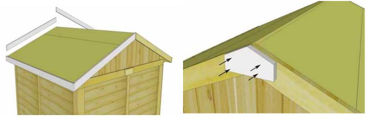
**57.** Complete remaining facia pieces. Attach **Pentagon Facia Plate** where Side Facia meet at the peak. Use 4 - 1 1/2" finishing nails per piece to secure.
