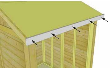
**56.** Position and attach **Front Facia** to ends of Roof Rafters with 10 - 1 1/2" nails. Front Facia will cap side facia in corners and line up on top edge with plywood roof.
