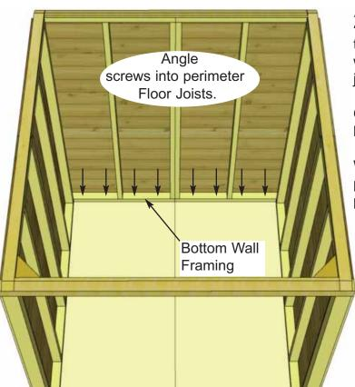
**27.** When all Walls and Top Plates are attached together, check wall and floor alignment. Bottom wall framing should sit flush with outside of floor joists. See **Steps 15-20** for correct alignment.
