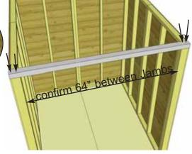
**23.** Position and attach the Door Header flush to outside end of Door Jamb with 2 - 2 1/2" screws per side. Important- Drill 1/8" pilot holes in end of Door Header to prevent wood from splitting.
