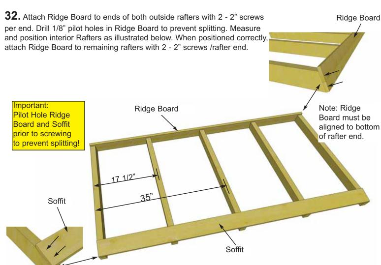
**33.** Attach end of Soffit Board flush to ends of outside rafters with 2 - 1 1/4" screws per rafter end. **Drill pilot hole in Soffit ends to prevent splitting.** Complete both outside Rafter / Soffit connections first. Measure and position interior Rafters as illustrated above. When positioned correctly, attach Soffits to remaining rafters with 2 -1 1/4" screws /rafter. Flip completed rafter section over.
