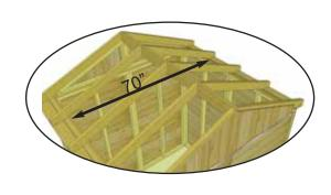
**41.** Secure Rafters to Top Wall Framing with one 3" screw per rafter. Screw through Wall Frame at an angle. Have two helpers push the Front and Rear Walls at the top from the outside of shed until inside to inside measurement between the Top Plates is 70".
