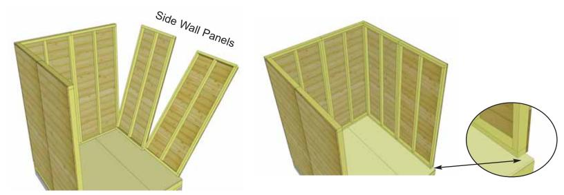
20. Position and attach remaining side wall panels together as per Steps 16-18.
