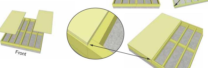
**10.** Position **Plywood Floor** pieces (2) on top of completed floor frames. The Plywood is cut slightly smaller than floor framing. Keep plywood seams tight.
