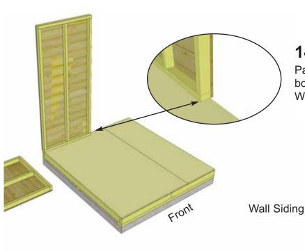
**14.** Starting at Rear Corner, position a Wall Panel on top of plywood floor. The Wall Panel bottom framing will sit flush with Floor Framing. Wall siding will overhang the floor.
