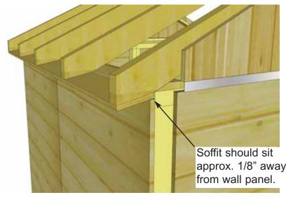
**37.** When Rafter Section is correctly positioned, outside rafters will sit equally on gable framing and Soffit will sit approximately 1/8" away from wall panels.
