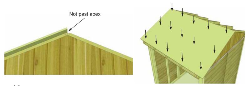
**44.** When Plywood is correctly positioned, fasten down into Roof Rafters with 15 - 1 1/4" screws.
