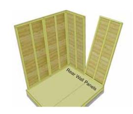
**18.** Align vertical wall studs of both side wall panels together and attach with 3 - 2 1/2" screws. Wall siding should overhang floor by approximately 1/2". Position 2nd rear wall panel as previously described.
