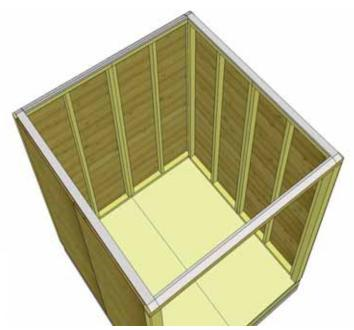
**26a.** Attach front Front Triangular Corner Brackets - 1 1/2" x 5 1/2" x 5 1/2" to header and wall frame with 2 - 2 1/2" screws per piece.
