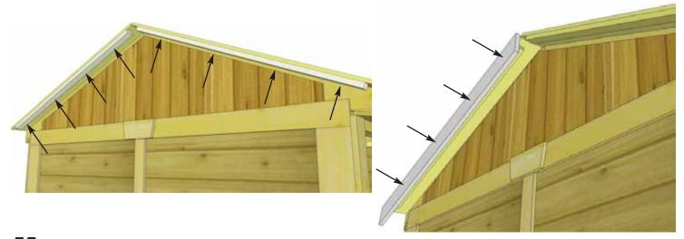
**55.** Attach **Facia Nailing Strips** (4 - 3/4" x 1 1/2" x 42") to underside edge of plywood roof with 4 - 1 1/4" screws per piece. Do this on both sides of the shed.
