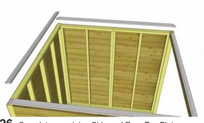
**26.** Complete remaining Side and Rear Top Plate attachments as per **Steps 24-25**.
