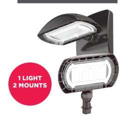
Commercial Electric's highly-versatile compact LED Flood Light with Wall Pack Mount Kit offers a wide range of security and architectural lighting applications. The fixture comes with two types of mounting arms: (1) a standard 1/2" swivel NPS floodlight mount for ground installations or wall and eave mounting, and (2) an angle-adjustable wall pack plate to transform the light into an architecturally stunning full-cutoff wall pack.
