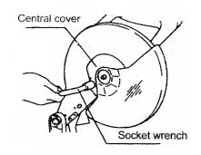
When removing the saw blade, first raise the handle to the highest position, press down the shaft-locking arm to lock the saw blade in place, and loosen the hex bolt by turning clockwise using the socket wrench. Then, remove the hex bolt, outer flange, and saw blade.
