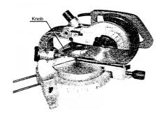
Release the knob in order to slip the carriage freely, completely pull the carriage towards the operator. Switch the machine on and wait until the saw blade reaches its maximum speed, then press the handle and push it to the cross bar in order to cut the work piece. Once you have finished cutting, turn the switch off and wait until the saw blade comes to a full stop, then raise the handle completely.
