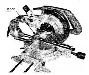
Push the carriage to the end towards the cross bar, tighten the knob to fix the carriage. Use the vise to secure the work piece. Switch the machine on, wait until the saw blade reaches its maximum speed, and then press the handle downwards slowly. After you have finished cutting, turn the switch off and wait until the saw blade comes to a complete stop before raising the handle completely.
