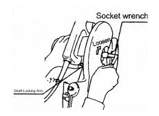
Install the new saw blade. Check that the teeth point in the direction of the arrow (see the protective cover).
