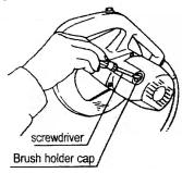
Use a screwdriver to remove the brush holder caps. Take out the worn carbon brushes, insert the new ones and secure the brush holder caps.
