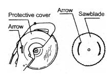
Install the outer flange and the hex bolt, then press down the shaft-locking arm, and tighten the hex bolt firmly by turning it counterclockwise using the socket wrench. Then secure the central cover back in place by adjusting the hex bolt. When removing the saw blade, lift up the movable hood and central cover, loosen the hex bolt with the socket wrench, remove the hex bolt, outer flange, and saw blade.
