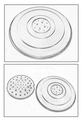
1. Grab the base of the fan as well as the internal base and prepare to attach.
