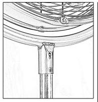
5. With help, attach the top of the fan to the fan base with the hardware provided.
