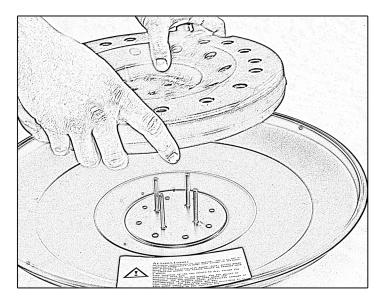
2. Attach the under part of the base to the outer part of the base with the provided screws, nuts, and washers.
