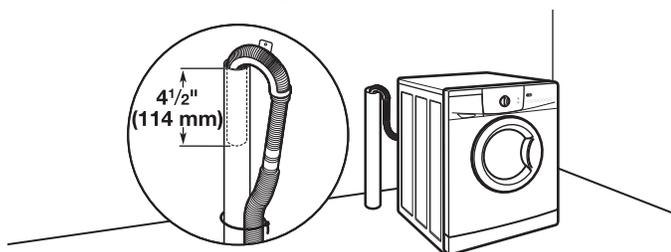
Minimum diameter for a standpipe drain: 2" (51 mm). Minimum carry-away capacity: 17 gal. (64 L) per minute. A 1/4" (6 mm) diameter to 1" (25 mm) diameter Standpipe Adapter Kit is available (Part Number 3363920). Top of standpipe must be at least 30" (762 mm) high; install no higher than 55" (1.4 m) from bottom of washer. If you have an overhead sewer and need to pump higher than 96 inches, a sump pump and associated hardware are needed. See "Alternate Parts".
