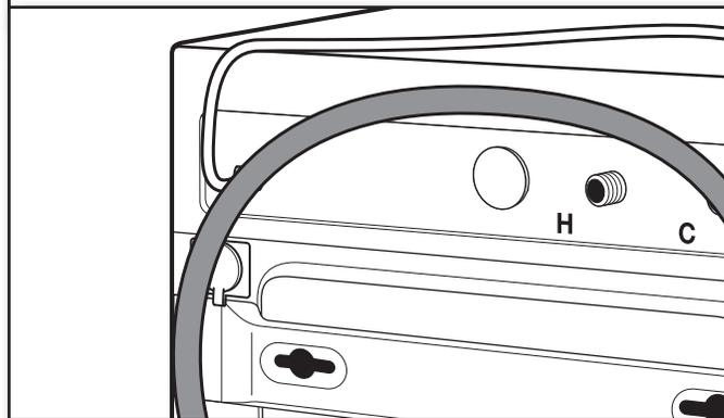
Remove the yellow shipping strap from the cord. Gently place power cord over top of washer to allow free access to back of washer.
