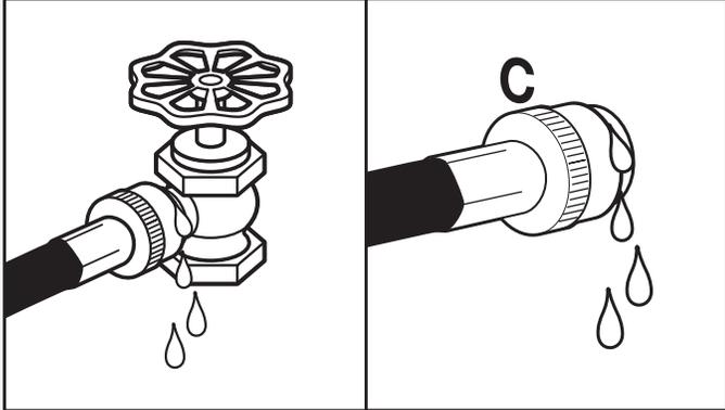
Slowly turn on water faucets to check for leaks. A small amount of water may enter washer. It will drain later.
