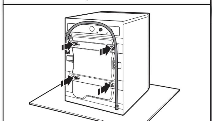
Locate four transport bolts on rear of washer.
