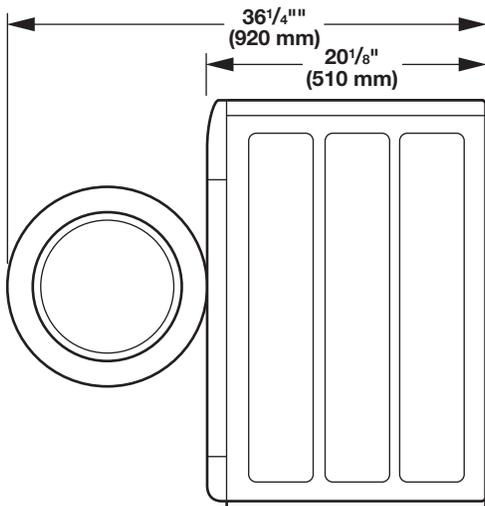
All dimensions show recommended spacing allowed, except for closet door ventilation openings which are the minimum required.
