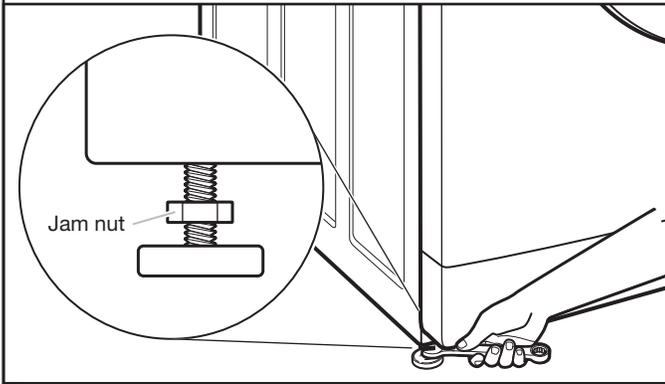
If washer is not level, use a 1/2" or 13 mm open-end or adjustable wrench to turn jam nuts clockwise on feet until they are about 1/2" (13 mm) from the washer cabinet. Then turn the leveling foot clockwise to lower the washer or counterclockwise to raise the washer. Recheck levelness of washer and that all four feet are firmly in contact with the floor. Repeat as needed.
