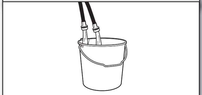
Run water for a few seconds through hoses into a laundry tub, drainpipe, or bucket to avoid clogs. Water should run until clear.
