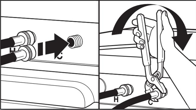
Attach hot water hose to hot water inlet valve. Screw coupling by hand until it is snug. Use pliers to tighten couplings an additional two-thirds turn. Repeat with cold water inlet valve.
