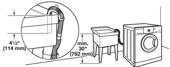
Minimum capacity: 20 gal. (76 L). Top of laundry tub must be at least 30" (762 mm) above floor; install no higher than 55" (1.4 m) from bottom of washer.
