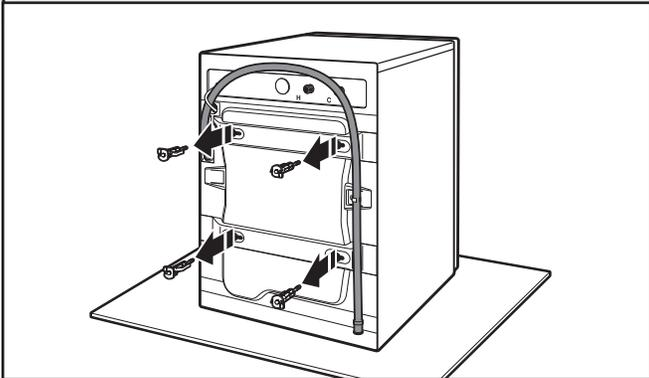
Loosen bolts with a 15/32" (12 mm) wrench. Once the bolt is loose, move it to the center of the hole and completely pull out the bolt, including the plastic spacer covering the bolt.
