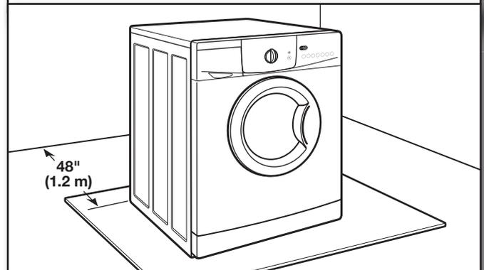
It is necessary to remove all shipping materials for proper operation and to avoid excessive noise from washer. Move washer to within 48" (1.2 m) of its final location. It must be in a fully upright position.
