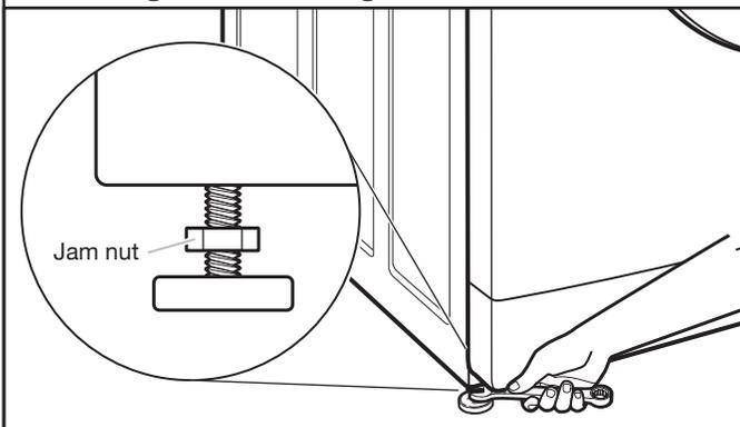
When washer is level and all four feet are firmly in contact with the floor, use a 15/32" or 12 mm open-end or adjustable wrench to turn jam nuts counterclockwise on leveling feet tightly against washer cabinet.
