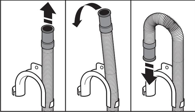
For floor drain installations, you will need to connect the drain hose form to the end of the drain hose. You may need additional parts with separate directions. See "Alternate Parts".
