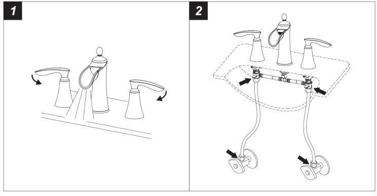
1. Turn the faucet handle all the way on, turn on hot and cold water supply and flush water lines for one minute. Reinstall aerator by hand.
