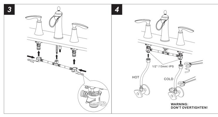
3. Position the flexible hose as shown and fix it to the faucet as shown with clamp spring.
