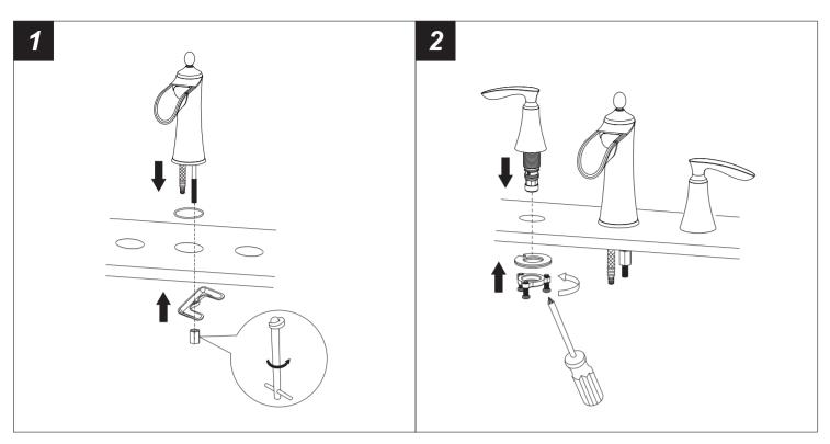
1. Position the body with o-ring in the installation surface as shown and secure it with metal washer and tighten the lock nut with basin wrench.
