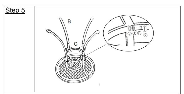
Loosely attach the Round Support (C) to Table Leg with pre-attached Leveller(B) with washers((2)),spring washers((3)) and hex nuts((5)) using spanner((7)).
