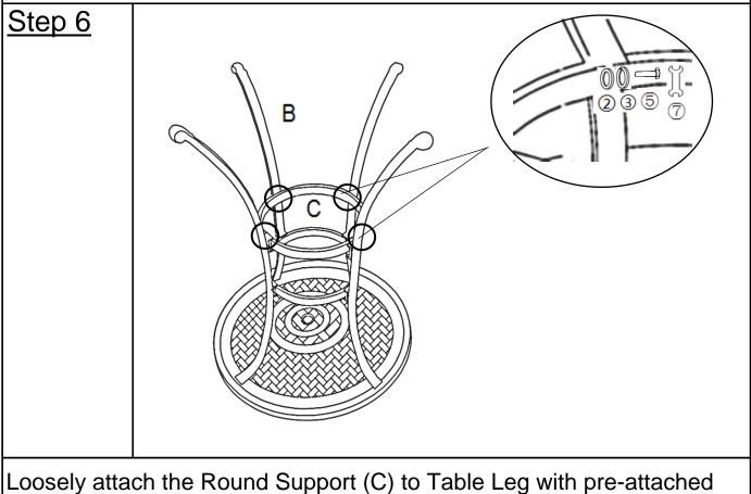
Loosely attach the Round Support (C) to Table Leg with pre-attached Leveller(B) with washers(2),spring washers(3) and hex nuts(5) using the spanner(7).
