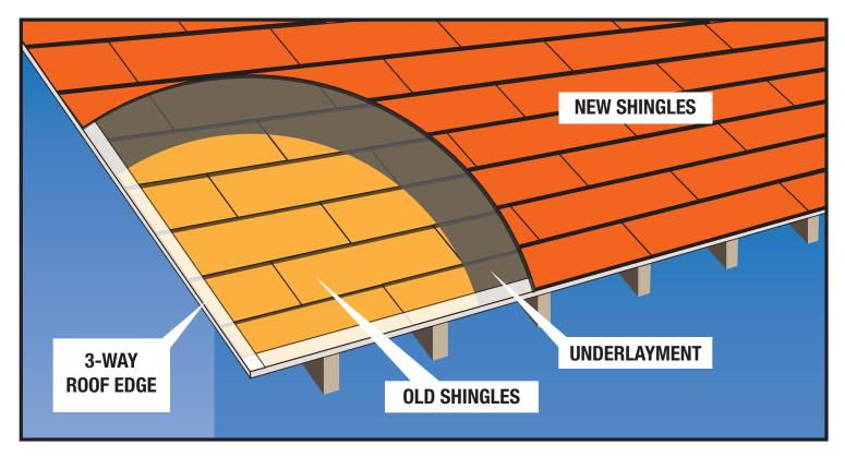
Recover: Applying a new, additional layer of shingles on top of an already existing shingle roof. Typically, the maximum number of layers allowed is two, on roofs with a 4/12 slope or less.
