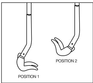
**NOTE:** Insert tool head fully under board for maximum lifting leverage.
