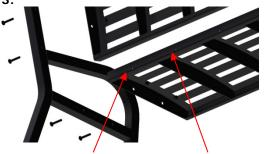
Note the water drain hole location on each seat section. For the Seat section, the holes should be facing the back of the bench when fastened to the bench ends.
