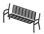
Using the supplied hardware (Items 3 & 4) and the supplied Phillips driver bit (Item 5), loosely assemble the Seat section (Item 1) to the (2x) Bench End Frames (Item 2). **Note:** This may be easier with two people.
