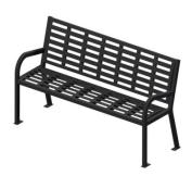
Verify all hardware is tightened (do not over tighten). Place the bench where you would like to permanently install, and mark the solid surface below the bench through the holes in the four feet. Using concrete anchors on a solid surface, drill a 3/8" diameter pilot hole 1-3/4" deep into the solid surface, and secure the bench to the ground using the supplied 3/8" hardware.
