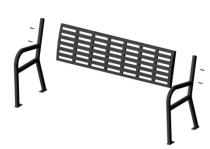
Using the supplied hardware (Items 3 & 4) and the supplied Phillips driver bit (Item 5), loosely assemble the back rest (Item 1) to the (2x) Bench End Frames (Item 2). **Note:** This may be easier with two people.
