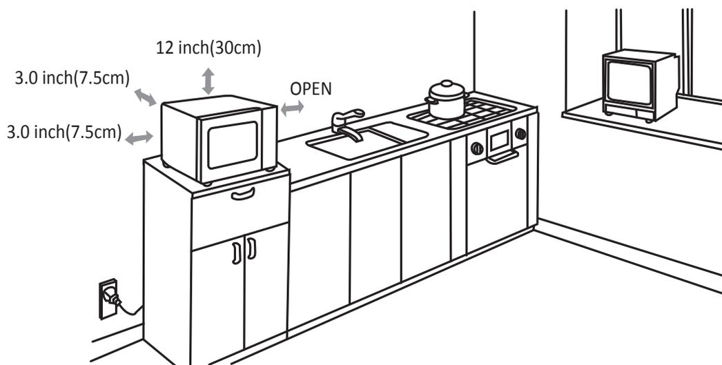
1. Select a level surface that provides enough open space for the intake and/or outlet vents. A minimum clearance of 3.0 inches (7.5cm) is required between the oven and any adjacent walls. One side must be open.
