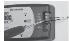
WiFi module. Turn the screw clockwise to secure the wire.
