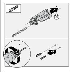
4) Install mounting plate (D2). Secure with two screws (E). Replace cradle mount cover (D1).
