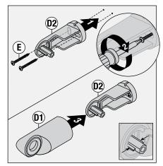
**Note:** Mounting plate (D2) center tabs must be horizontal for installation.
