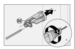
**Option:** Place mounting plate (D2) in position, mark and drill 3/16" holes into wall. Install anchors.
