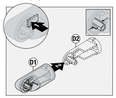
**Note:** Mounting plate (D2) center tabs must be horizontal for removal.
