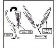
For an inside mount installation, insert the valance clips into the valance groove located on the backside of the valance. Afterwards, make sure the valance clip is securely fastened to the headrail before using your blind.
