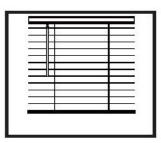
Hold Down Brackets(Optional) Using two small screw, screw hold down bracket to window or wall . Snap bracletpin ends into the hole at the bottom rail end.
