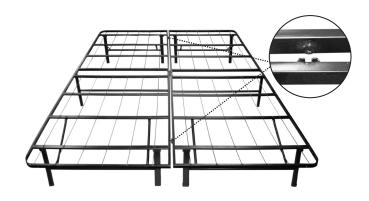
**Step 5.** Insert two halves together with keyhole locked in place.
