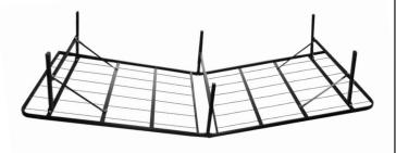
Step 2. Unfold each half and lay flat. Raise all six legs to upright position. Each of the four end legs have separate support arms. Rotate support arms to hook on to the bolts and tighten with installed wing nuts. Note: The two center legs do not require wing nuts.
