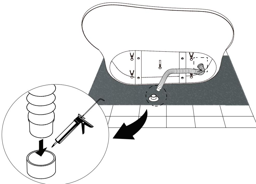
12. Apply silicone along the bottom of the bathtub in order to create an airtight seal. Then apply a bead of tub & tile caulk around the edges of the base.
