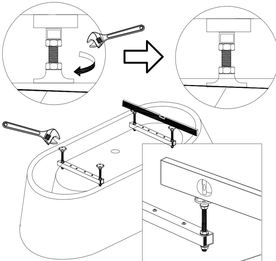
7. Ensure to mark all positions of leveling legs on the floor using a pencil. Move the bathtub into the desired location near the drainpipe.
