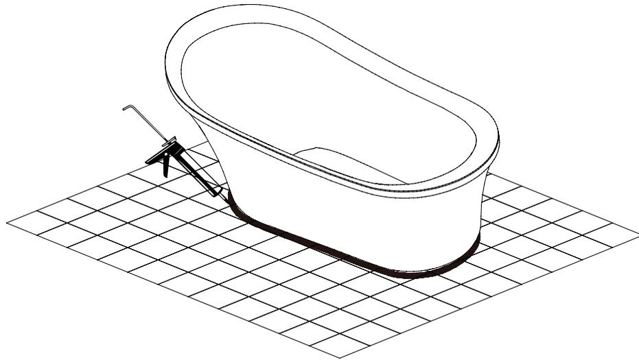
13. With the bathtub now in place, wipe off any excess silicone, tub & tile caulk where the bathtub meets the floor.
