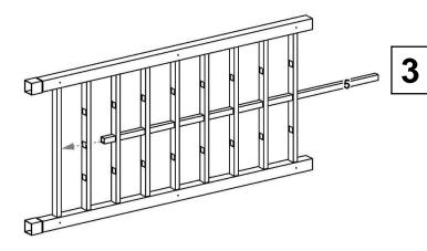
Insert 58" vertical rail (part 5) through center hole of cross rails.
