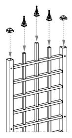
Using PVC, super or crazy glue, glue post caps onto posts and arrowhead caps onto vertical rails.
