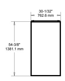
MATERIALS: 1/8" (3.175mm) Tempered Glass Panels with pre-assembled Anodized Aluminum Frame
