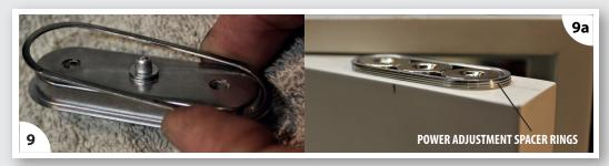
Remove the **DOOR MAGNETIC ASSEMBLY** from the top of door, turn the assembly over and fit (1-5x) **POWER**
