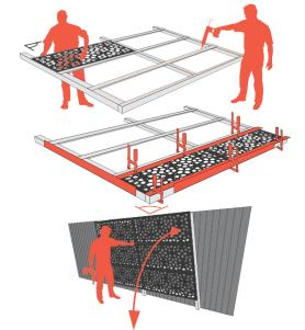
Prefabricating multiple panels to a frame is one effective way to install.
