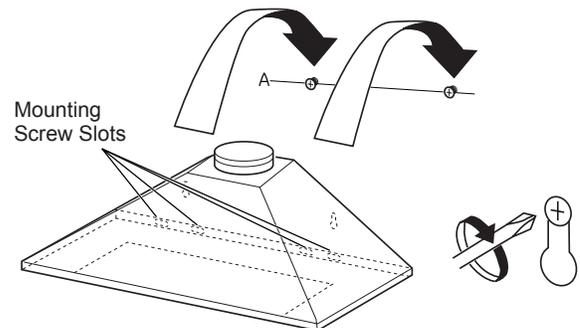
2. Insert 2 mounting screws into the 2 duct cover anchors (installed on line D in Preparing the Wall section) located in the slots on the back surface of the hood. Secure tightly.
