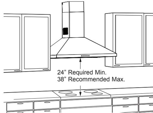
The vent hood must be installed between the 24" required minimum and 38" recommended maximum above the cooking surface. The hood installation height above the cooking surface depends upon ceiling height and duct cover limitations. The telescopic duct cover conceals the ductwork running from the top of the hood to the ceiling. For supplied duct cover ceiling heights, see table on page 5.
