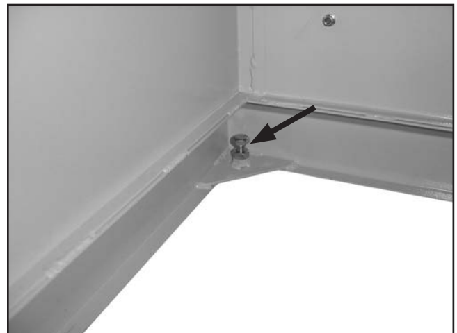
Figure 16. Hex bolt in stand corners for leveling; the hex nut is used to secure bolt position.
