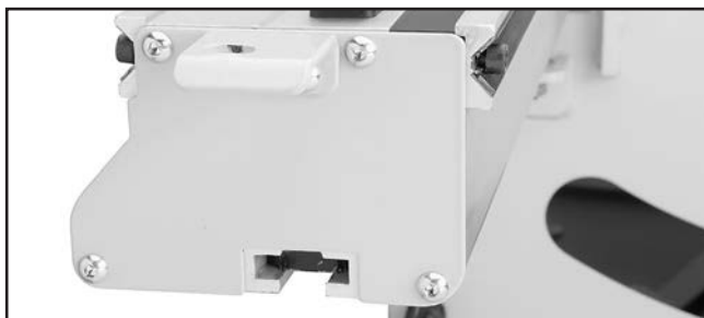
Figure 33. Sliding table end cover installed.
