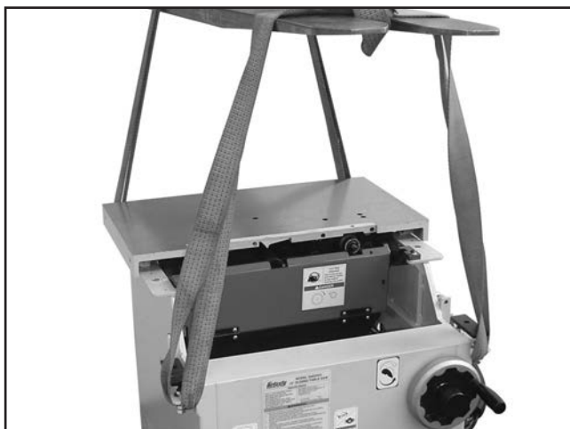
Figure 15. Lifting the table saw cabinet.
