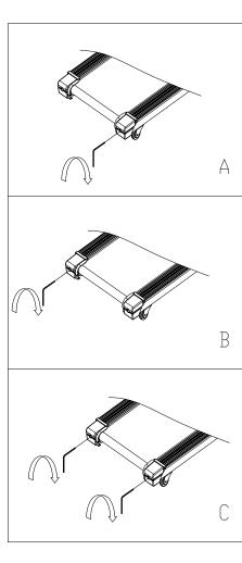
Place the treadmill on flat ground, set running speed to about 6-8km/h and watch the running belt deviations.
