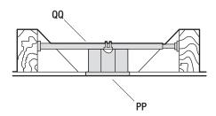
To hang your fan where there is an existing fixture but no ceiling joist, you may need an installation hanger bar (QQ) (not included) as shown above.
