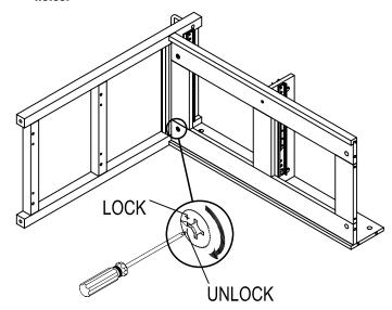
Wood dowel Cam lock bolt Cam lock Small head Large head
