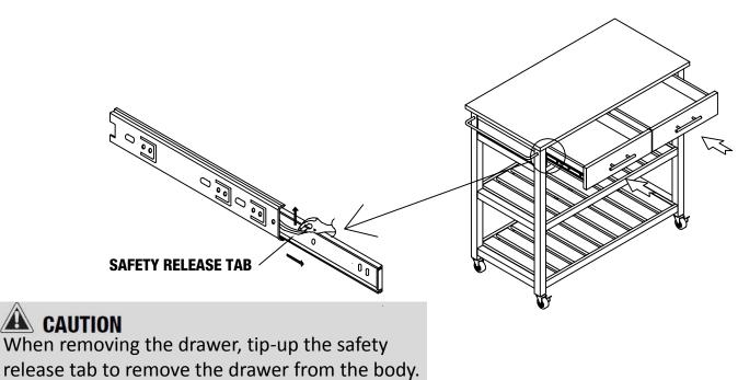
release tab to remove the drawer from the body.
