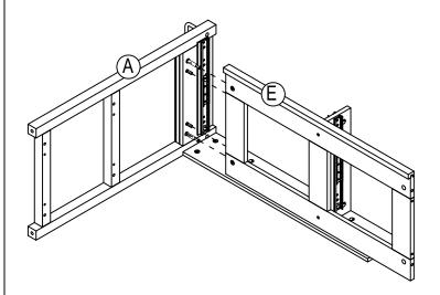
$\ \Box$  **d)** Tighten bolt (FF) with lock (GG) in the pre-drilled holes.
