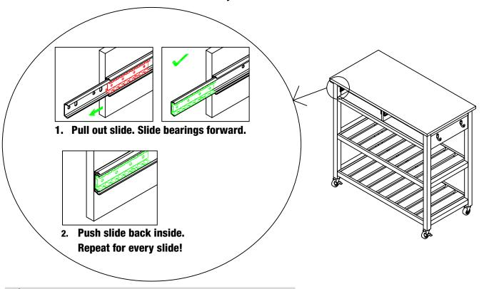
Make sure the slide piece is at the front end of the glide when installing the drawer into the body.
