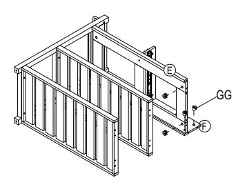
□ **C) Join** frame (**B**) to the assembled body with dowel (**EE**).
