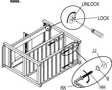
e) Install washer (JJ), washer (II) and bolt (HH) in turn as shown, tighten the bolt (HH) with wrench (KK).
