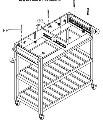
□ **C)** Join panel (J) to the assembled body with dowel (EE) first.
