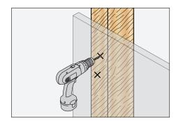
Align mounting holes on Grab Bar with drill holes. Insert wood screws into pilot holes for wall and wall studs. Hand tighten wood screws.
