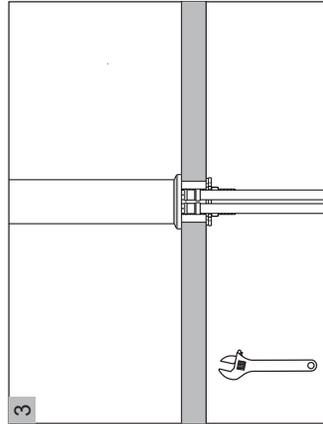
**3** If necessary, tighten screws using an adjustable wrench until the faucet is firmly connected to the sink.
