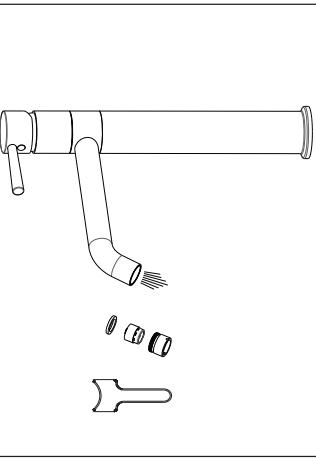
After installation is complete, remove aerator and rotate handle to the closed position. Turn on the water supply valves, and check all connections for a leak. Turn on your faucet and allow both hot and cold water to run at least one minute each. Replace Aerator.
