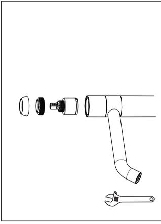
Remove handles. Unscrew Dome Cap counter clockwise by hand. Unscrew Retaining Nut using adjustable wrench, take out cartridge assembly and inspect. Replace parts as necessary. Reassemble parts by reversing steps.
