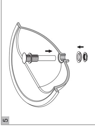
**5** Unscrew Locknut. Make sure the Rubber Washer in the right position under Flange. Insert Pop-up Assembly into Sink drain Hole. From underneath, tighten with Lockset.
