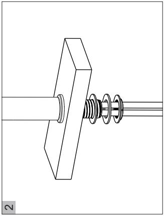
Install without Deck Plate. Make sure the O-RING is placed onto the bottom of Base Ring. Install faucet through hole in sink. From underside sink, put Plastic Washer and Mounting Nut. Position faucet on sink properly and tighten Mounting Nut.
