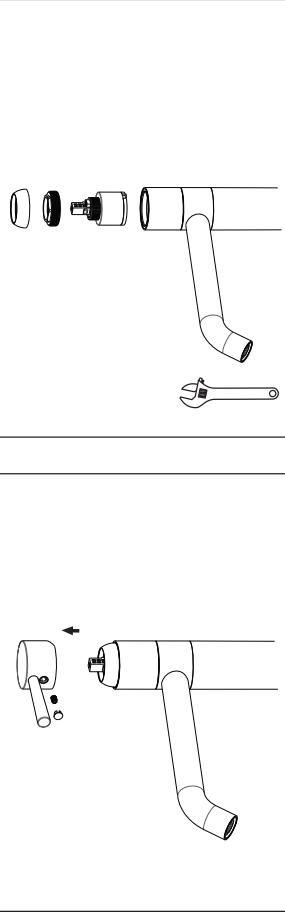
Turn off water and relieve pressure! Detach handle button using a small flathead screwdriver, unscrew set screw using Allen Wrench and take off handle.
