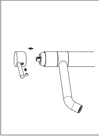
Turn off water and relieve pressure! Detach handle button using a small flathead screwdriver, unscrew set screw using Allen Wrench and take off handle.
