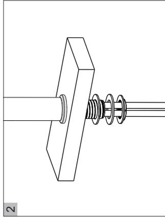
**2** Install without Deck Plate. Make sure the O-RING is placed onto the bottom of Base Ring. Install faucet through hole in sink. From underside sink, put Plastic Washer and Mounting Nut. Position faucet on sink properly and tighten Mounting Nut.
