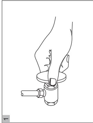
**1** You should clean all the dirt from valve outlets. Turning off the water supply valves. This is usually found near the water meter. If you are replacing an existing faucet, remove the faucet from the sink and clean the sink surface thoroughly.
