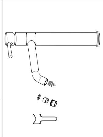
After installation is complete, remove aerator and rotate handle to the closed position. Turn on the water supply valves, and check all connections for a leak. Turn on your faucet and allow both hot and cold water to run at least one minute each. Replace Aerator.
