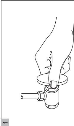
You should clean all the dirt from valve outlets. Turning off the water supply valves. This is usually found near the water meter. If you are replacing an existing faucet, remove the faucet from the sink and clean the sink surface thoroughly.
