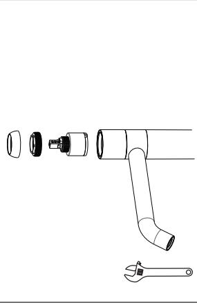
Remove handles. Unscrew Dome Cap counter clockwise by hand. Unscrew Retaining Nut using adjustable wrench, take out cartridge assembly and inspect. Replace parts as necessary. Reassemble parts by reversing steps.
