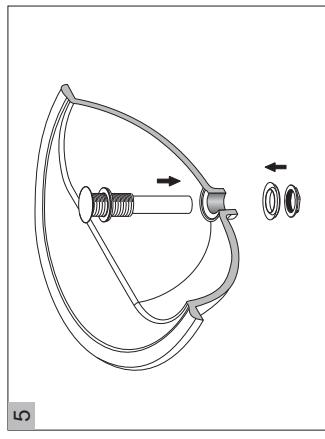
Unscrew Locknut. Make sure the Rubber Washer in the right position under Flange. Insert Pop-up Assembly into Sink drain Hole. From underneath, tighten with Lockset.
