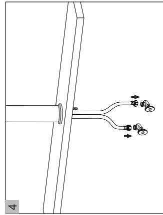
Connect hot and cold water supply lines to the Water Supply Valves.
