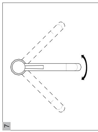
Lift the handle up, the cartridge will be activated allowing water to flow. The water flow will increase by continuing to rotate handle. By rotating the handle to the left, the water temperature will decrease to cold flow only. By rotating Handle to the left, the water temperature will increase to hot only.
