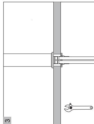
If necessary, tighten screws using a adjustable wrench until the faucet is firmly connected to the sink.
