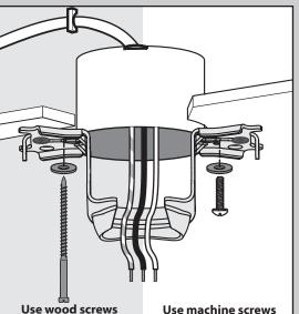
(included) when securing to support structure with approved electrical outlet box. Drill 9/64" pilot holes in support structure to aid in securing ceiling bracket with hardware found in the ★ hardware bag.
