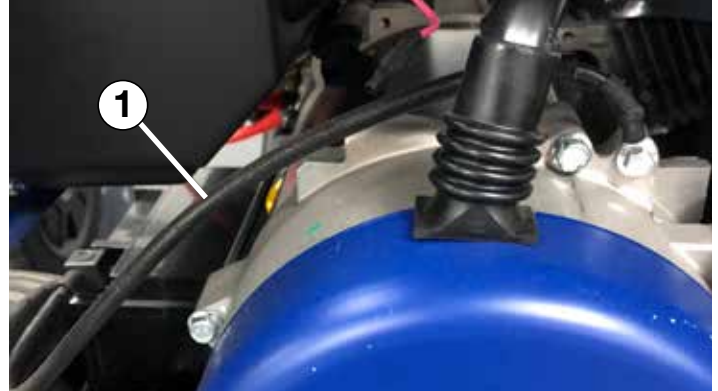
Figure 5 - Locating Negative (-) Cable
