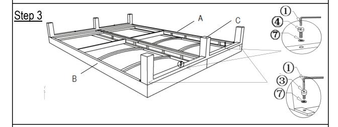
Repeat the process from **Step 2** to assemble the other Bed Leg(C). **Do not fully tighten the Bolts.**
