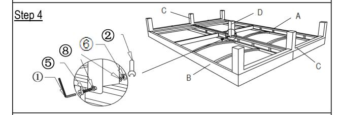
Attach Middle Leg(D) to Double Bed using Bolt(5) and Washer(8) on one side and Washer(8) and Nut(6) on the other side with Allen Key(1) and Wrench(2) as shown in the picture. **Do not fully tighten the Bolts.**
