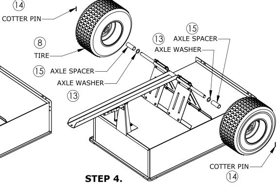
4. Slide axle washer and axle spacer over each side of axle as shown. Add wheels making sure valve stem faces out. Insert cotter pin in axle and lock in place by spreading ends. Turn cart upright and add tailgate.
