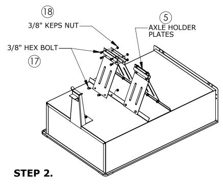
2. Loosely attach the four axle holder plates with the 3/8"x 3/4" hex head bolts provided. NOTE: these bolts will be tightened after axle and wheels are installed in a later step.
