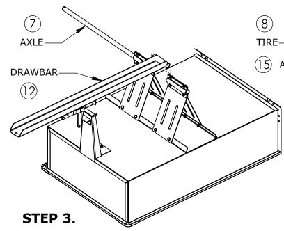
3. Center drawbar tube between axle holder plates and insert axle, making sure to center axle so that wheels can be put on in the next step.
