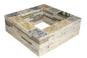
**Step 4**: Install the remaining 7 rows. Place the blocks in the same manner as Step 2 for each row staggering the joints of the blocks below. After making any adjustments to each row, remove one block at a time and glue to the two blocks below using a quarter sized dabs of construction adhesive. Installation is complete – Enjoy!
