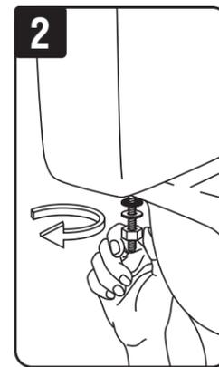
Unbolt tank from bowl, then lift tank and set on a stable, soft surface. Remove any remaining rubber washer, hex nut and bolts.
