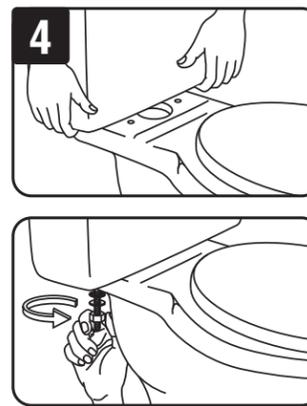
Before replacing the tank on the bowl, place metal washer and hex nut onto bolt under tank and hand tighten hex nut. Then place tank back on the bowl gasket so that tank to bowl gasket fits evenly. Level tank. Under the bowl attach rubber washer, metal washer and metal hex nut. Tighten the hex nuts under the bowl evenly until the tank is stable and doesn't rock. **DO NOT OVERTIGHTEN** or the tank or bowl could break.
