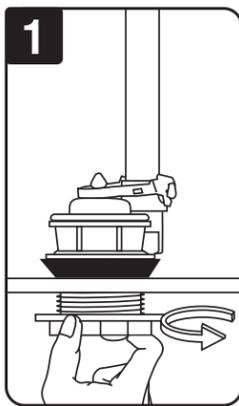
Place flush valve in tank. Position the overflow pipe toward the back of the tank. Do not cover bolt holes. Hand tighten flush valve lock nut. **DO NOT OVERTIGHTEN** or tank may crack.
