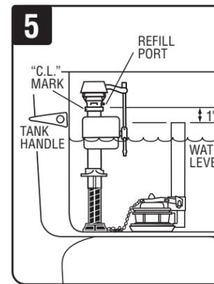
When installed the top of the overflow pipe of the flush valve must be at least 3" below the top of the fill valve.
