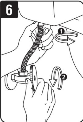
Reconnect water supply line to bottom of fill valve (1). Turn on water supply and check for any leaking. If leaking, turn nut just enough to stop leaking. Then flush toilet to check.
