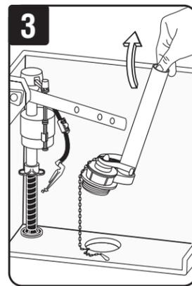
Remove tank-to-bowl gasket and large nut from old flush valve. Then remove flush valve from tank.
