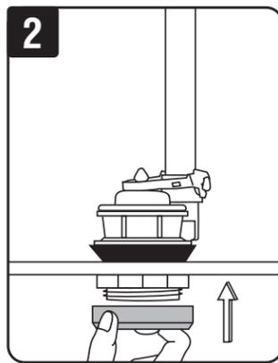
Slide new tank to bowl gasket over nut with narrow side facing down. Gasket should cover the nut completely.
