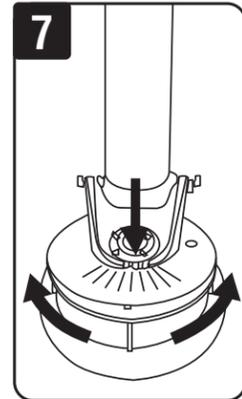
The higher the setting the longer the flush. To adjust flapper, rotate left or right to get desired flush. Factory setting is at maximum.
