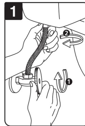
Turn off water supply (1). Flush toilet and remove excess water from tank with sponge. (2) Place bucket or towel under water supply line and remove nut of water supply line from bottom of toilet fill valve.
