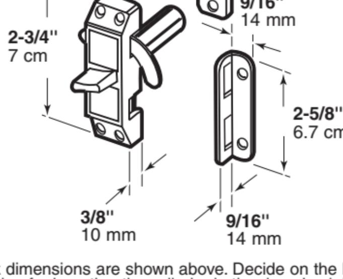
Lock dimensions are shown above. Decide on the hole position for inserting the cylinder in the door. Lock housing must be as close as possible to the jamb (see Figures. 1 & 2).
