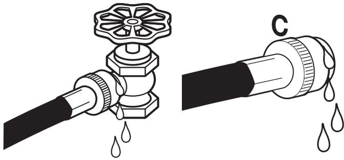
**NOTE:** Replace inlet hoses after 5 years of use to reduce the risk of hose failure. Record hose installation or replacement dates on the hoses for future reference.
