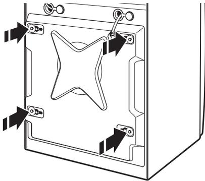
3. Once the bolt is loose, move it to the center of the hole and completely pull out the bolt, including the plastic spacer covering the bolt.
