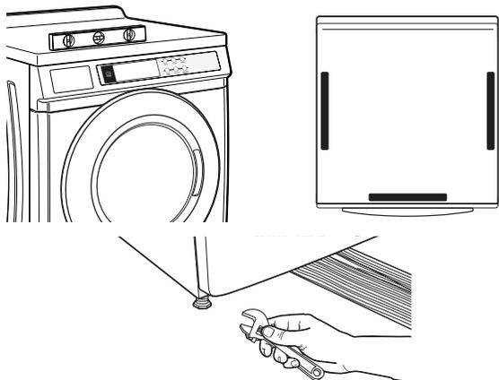
If the washer is against a wall, move the washer out slightly before tipping back. If the washer is not level, first prop the front with a wood block and adjust the feet as necessary; then prop the back and adjust feet as necessary. Repeat this step until washer is level.
