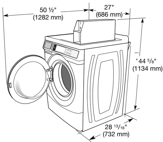
\*Height without leveling feet installed.
